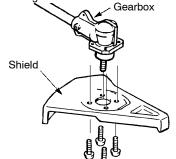
Insert the 4 mounting screws through the bottom of the shield. Thread them into the gearbox. Tighten evenly and securely with one of the hex key wrenches provided.
